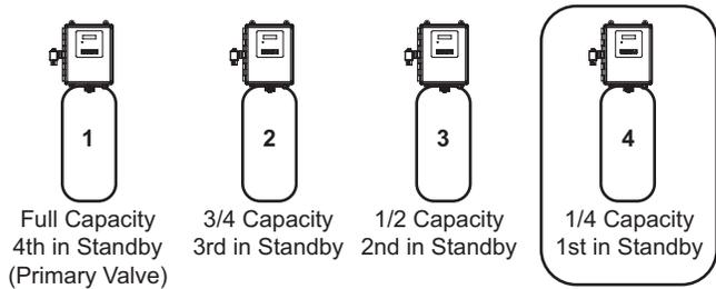
7. The primary tank regenerates. The next tank with the least remaining volume becomes the new primary tank. The tank with the next least volume remaining will be the first trip point programmed rate. Tanks continue operating in this order.
