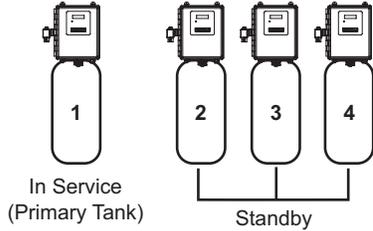
2. The total flow rate to the primary tank increased past the first trip point programmed rate. The flow stayed past the trip point delayed time. The next tank (least volume remaining) changes from Standby to In Service. This then splits the total flow between two meters.
