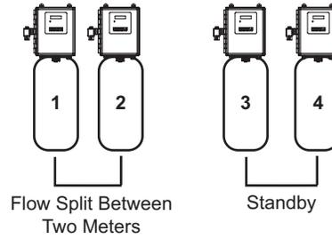
6. Tanks return to Standby due to decreased total flow rate and trip points programmed. The tank with the most remaining volume will be the first to go into Standby.
